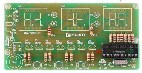
Step 6:Install 2pcs 30pF Ceramic Capacitor at C2,C3.
